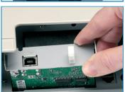
Easily Interchangeable interfaces-USB, Bluetooth, LAN, Serial, Parallel, WLAN, CloudPRNT, AirPrint, and WebPRNT\*
